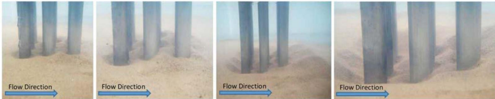
(a) single pile scour (b) dunes appear (c) dunes move backward (d) pile groups scour as whole
